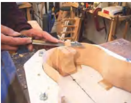
▲ Pic.30 Wedges are cut flush
